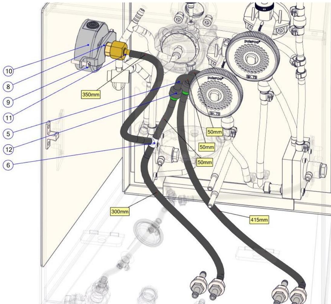
**AIR TUBES – VENT MECHANISM TANKS**
