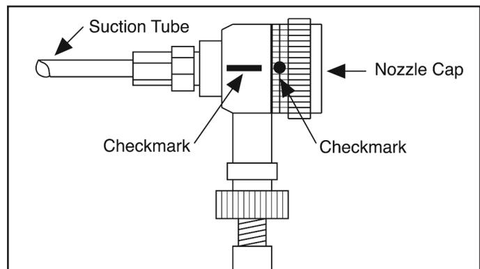
**WARNING:** The standard model Autofog uses a nozzle that is manufactured with brass components. The use of oxidizers will damage this nozzle within several applications.
