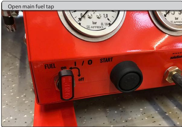
3.7. Open the fuel tap on the control panel setting it to the "ON" position (vertical).
