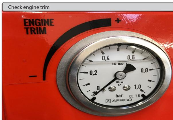
3.9. After the engine starts readjust the carburetor setting on the auxiliary carburetors. To obtain the maximum performance from the pulsejet engine on the K-50 try to set the auxiliary carburetors in order to maximize the pressure on the "engine trim" pressure gauge.
