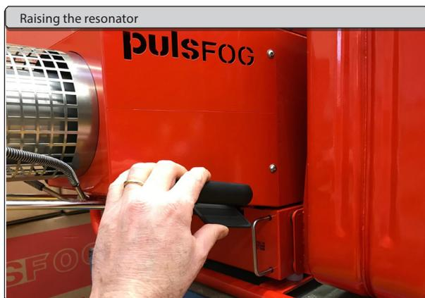
4.2. Raise the resonator to the desired inclination. Push button under the handle and raise the resonator manually to the desired position!
