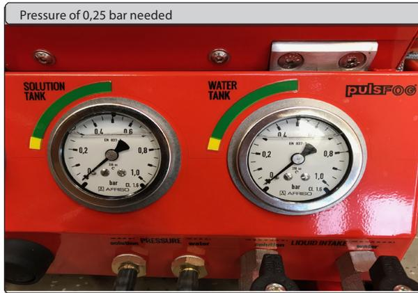
4.3. After up to two minutes after the engine start the formulation tank and the water tank should reach the pressure of at least 0.25 bar, which is the minimum pressure for fogging.
