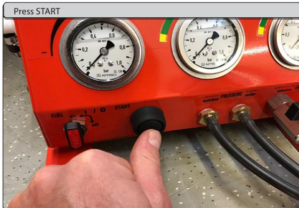
3.8. Press the "START" button for two seconds each time, pausing 3-5 seconds before pressing again, until the engine starts.
