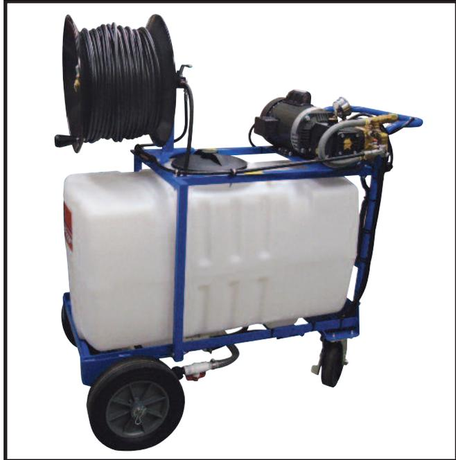
The motor has a 15.6 amp self-resetting thermal overload protection cut off. In the event of an overload, voltage drop, or over heating- the motor automatically shuts down. After a period of 3 - 4 minutes the pump can be turned on safely. The 10 foot main power cord is grounded. If you use extension cords, they should be #12 gauge grounded cords- and should not exceed 50 feet.
